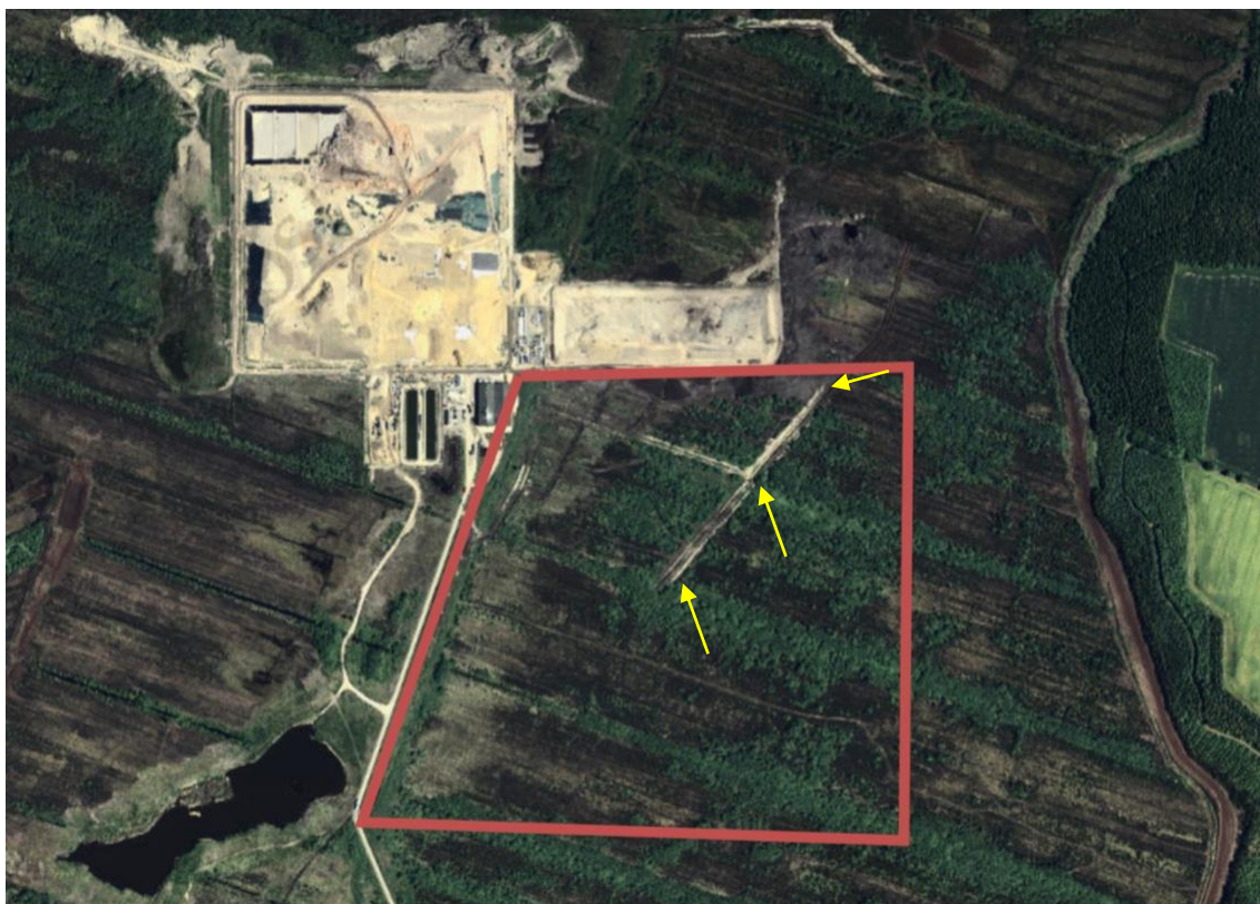
Figure 7 - MapGenie (2013- 2018) satellite image (Geohive, 2023) showing proposed site outlined in red and existing Phases 1 to 8 undergoing filling and capping and Phases 9 and 10 under construction. Diversion drain shown by yellow arrows.
